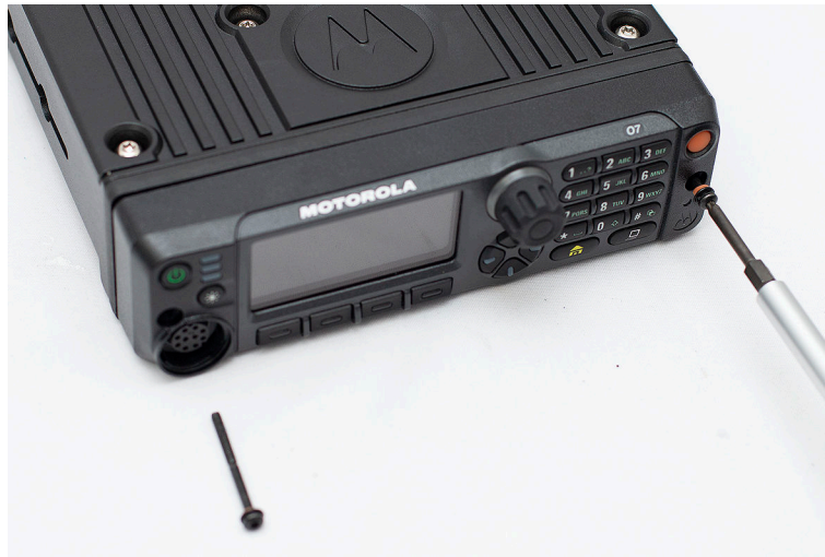
Figure 113: Attaching the Transceiver Screws
