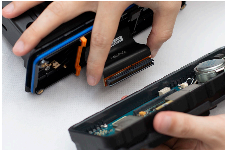
Figure 58: Disconnecting the Transceiver Flex from the Front Housing Assembly
