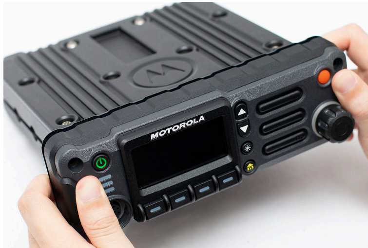
Figure 105: Attaching the Front Housing Assembly to the Back Housing Assembly
