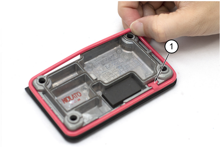
Figure 100: Inspecting and installing Bottom Cover Seal onto the Bottom Cover
