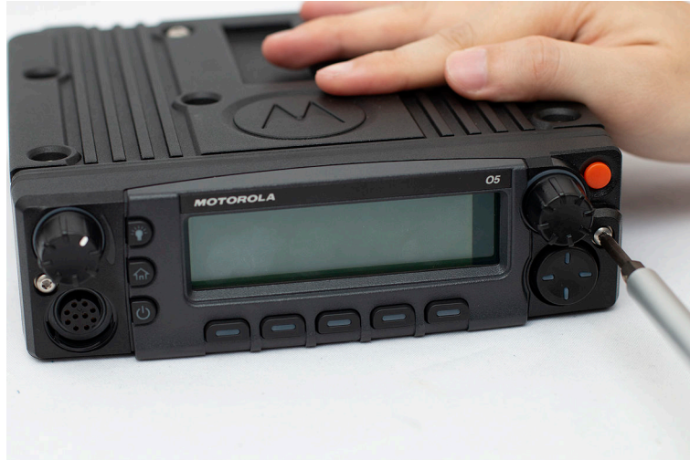
Figure 109: Aligning Control Head/TIB Front of Chassis, and Installing the Control Head/TIB Screws
