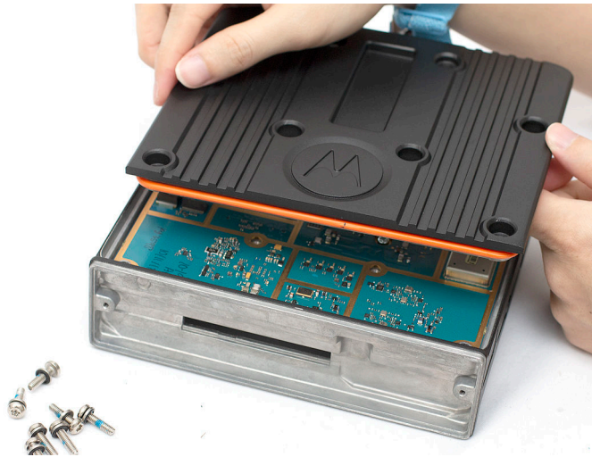
Figure 47: Removing the PA Screws
