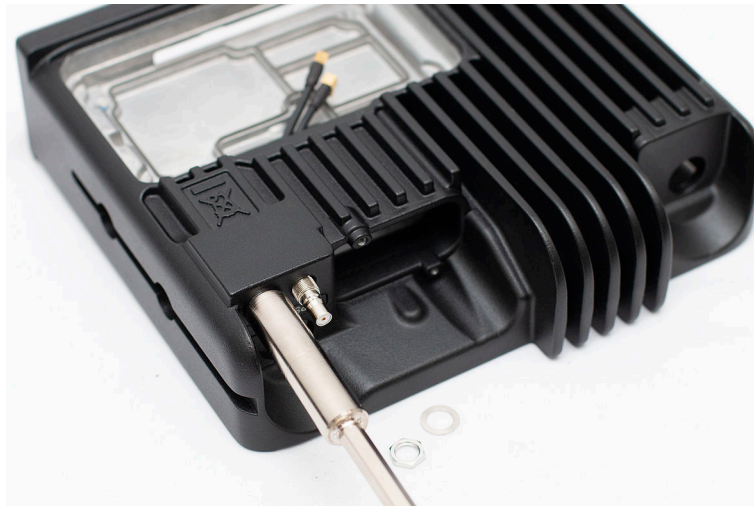
Figure 54: Removing the Wi-Fi QMA connector
