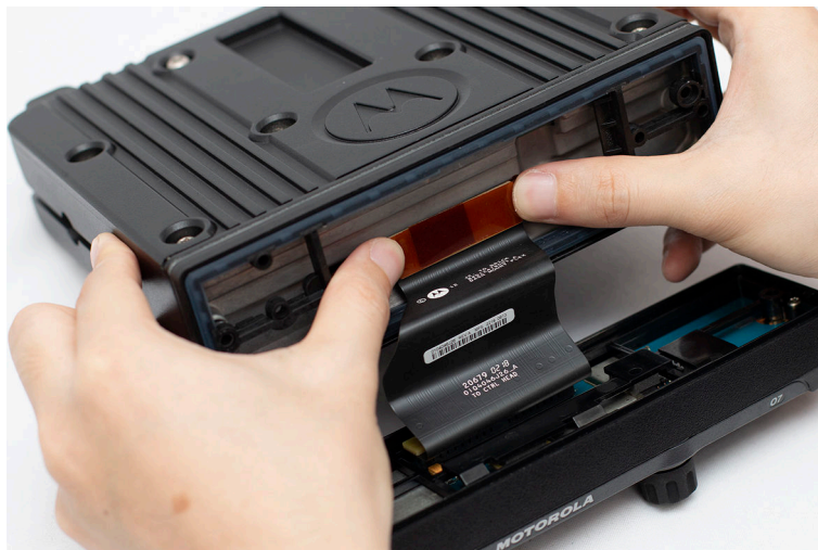
Figure 112: Attaching the Control Head to the Transceiver
