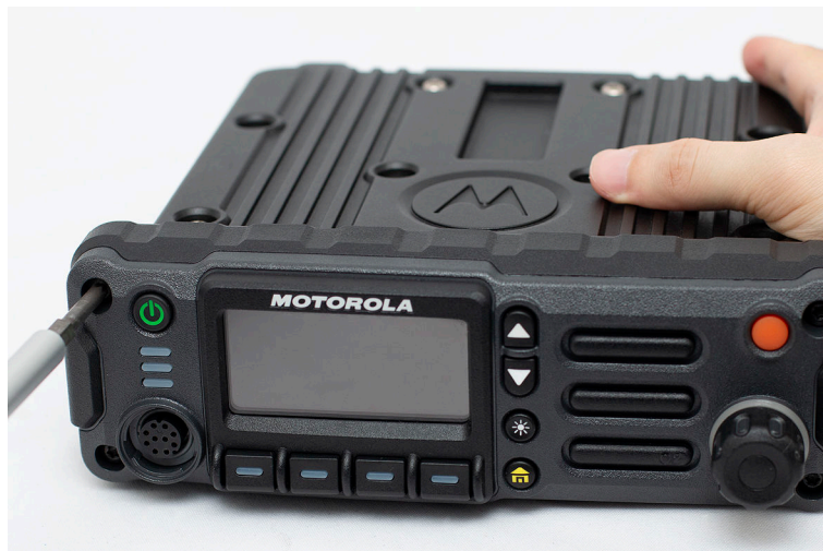
Figure 106: Attaching the Control Head Screws
