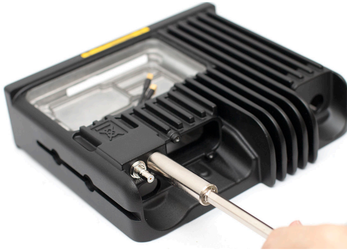
Figure 54: Removing the Wi-Fi QMA connector
