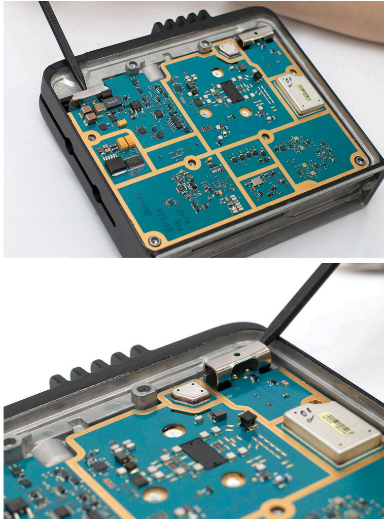
Figure 48: Removing the RF/DC Retention Clips
