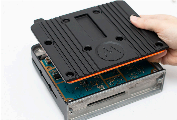
Figure 95: Placing the RF Cover onto Chassis
