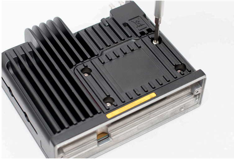
Figure 39: Removing the Bottom Cover Screws
