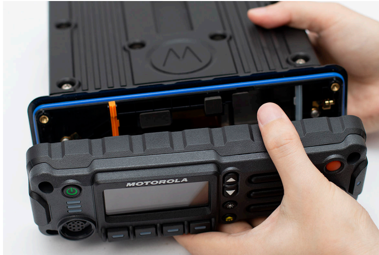
Figure 57: Removing the Control Head
