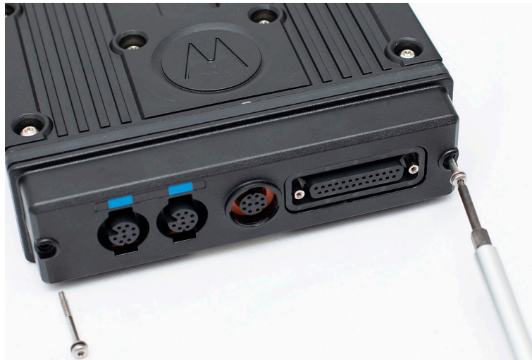
Figure 80: Removing the TIB Screws
