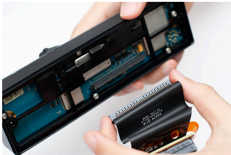
Figure 67: Removing the Transceiver Flex
