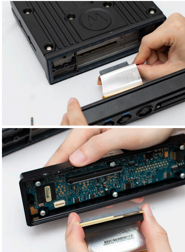
Figure 82: Removing the Flex
