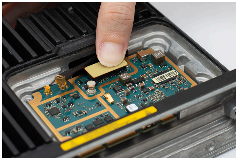
Figure 98: Installing Accessory Flex Connector to the Controller Board
