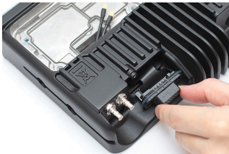
Figure 52: Removing the Rear Connector Flex
