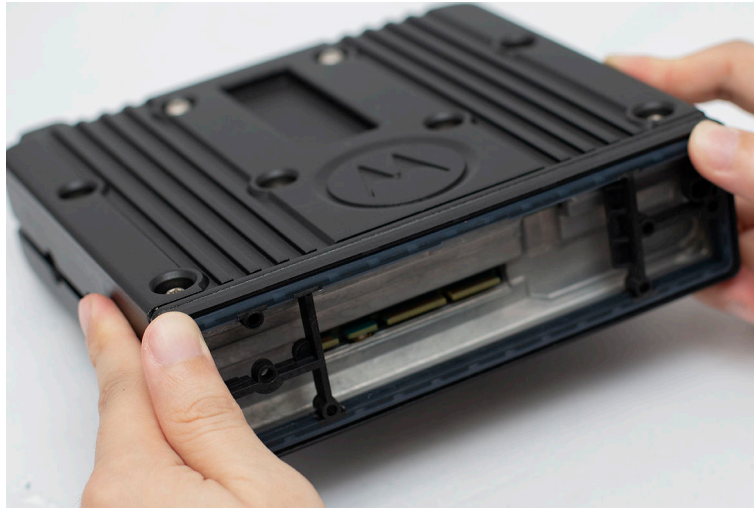
Figure 111: Attaching the I-seal to the Control Head
