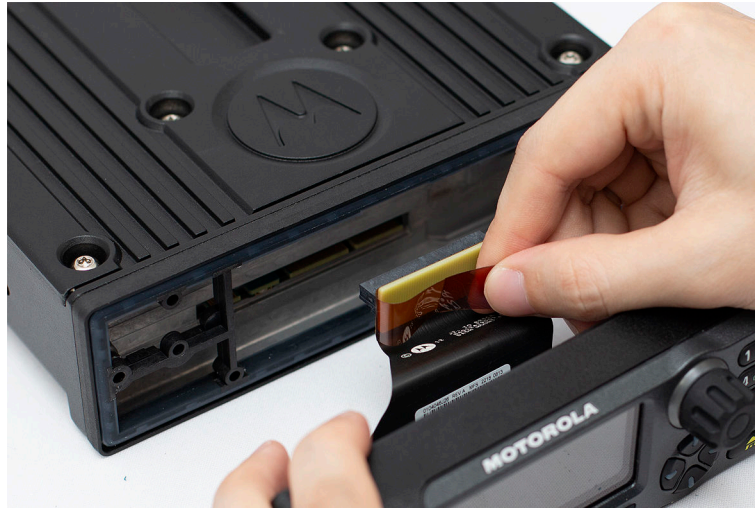
Figure 66: Disconnecting the Transceiver Flex from the Transceiver
