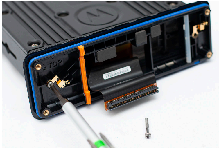
Figure 59: Removing the Back Housing Assembly
