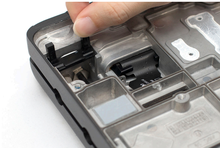
Figure 50: Removing the plastic retainer
