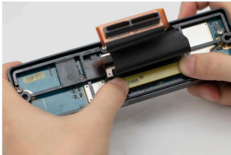
Figure 110: Installing the Transceiver Flex onto the Control Head
