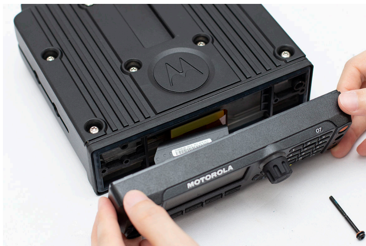
Figure 65: Removing the Control Head
