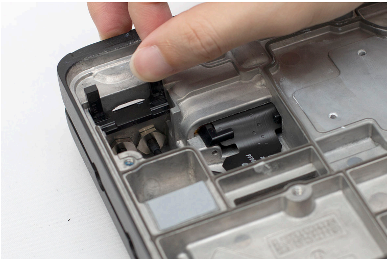
Figure 90: Placing the Plastic Retainer
