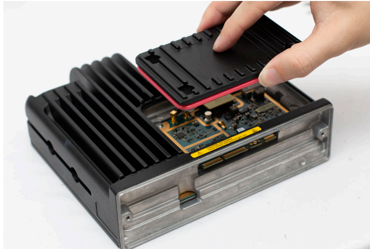
Figure 101: Placing Controller Cover on the Chassis
