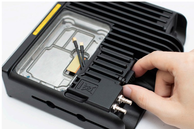
Figure 86: Inserting Rear Accessory Flex
