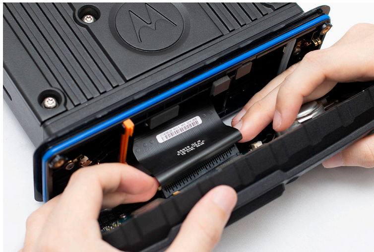
Figure 104: Installing the Transceiver Flex onto the Front Housing Assembly
