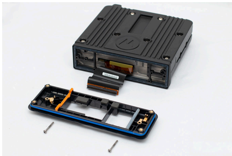
Figure 60: Removing the Transceiver Flex
