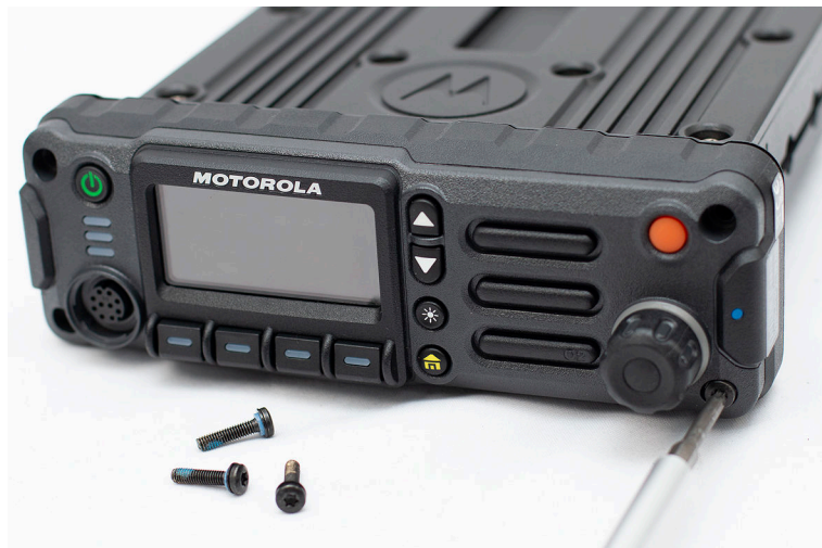
Figure 56: Removing the Control Head Screws
