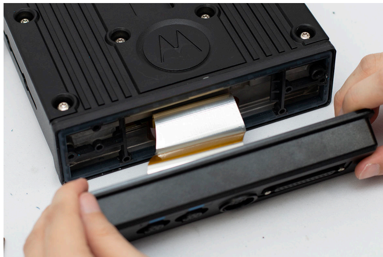
Figure 81: Removing the TIB
