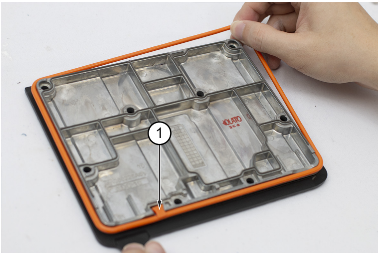
Figure 94: Inspecting and Installing the RF Cover Seal
