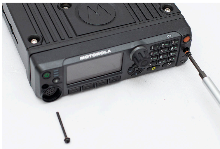
Figure 64: Removing the Transceiver Screws
