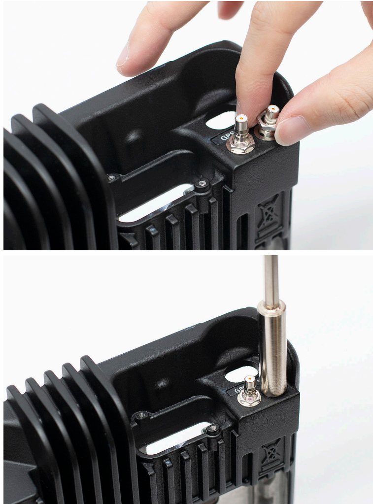
Figure 85: Inserting the GPS and Wi-Fi Cable
