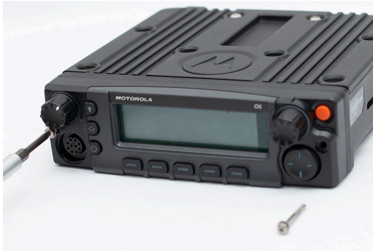
Figure 61: Removing the Control Head Screws
