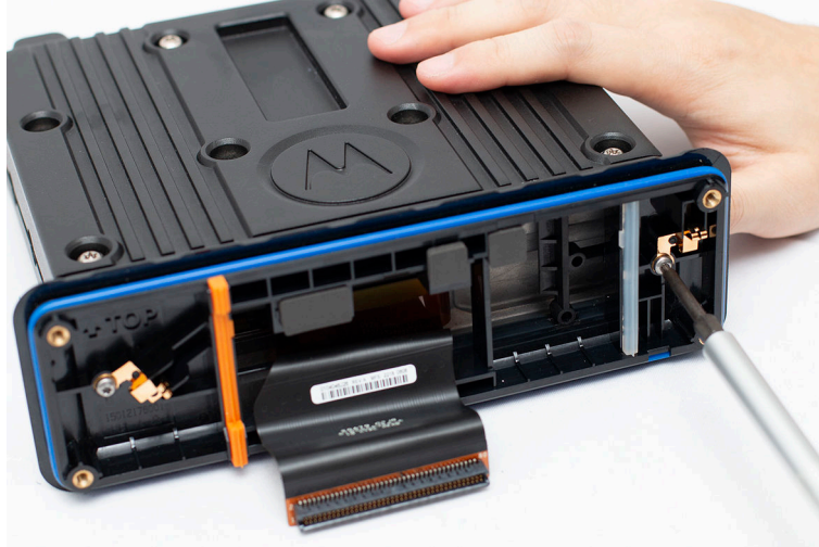
Figure 103: Installing the Back Housing Assembly onto the Transceiver
