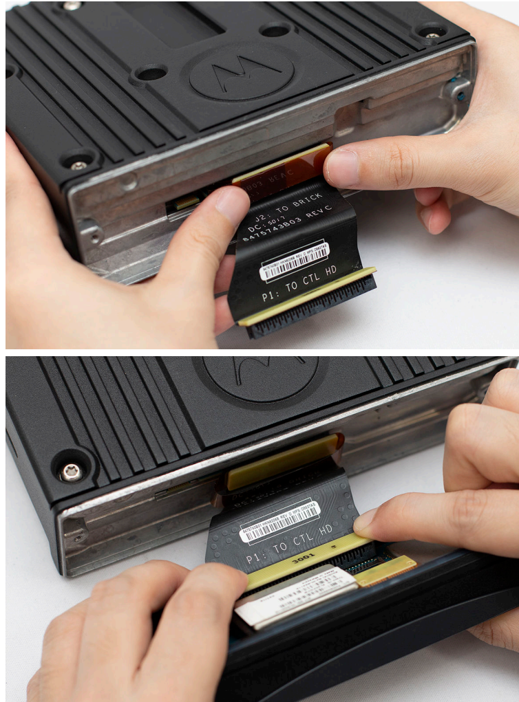
Figure 107: Installing Flex into the Controller PCB
