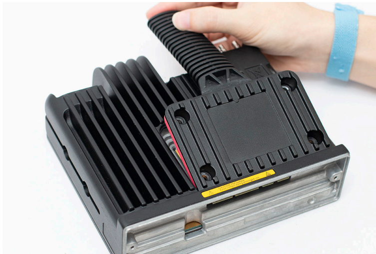
Figure 40: Removing the Bottom Cover
