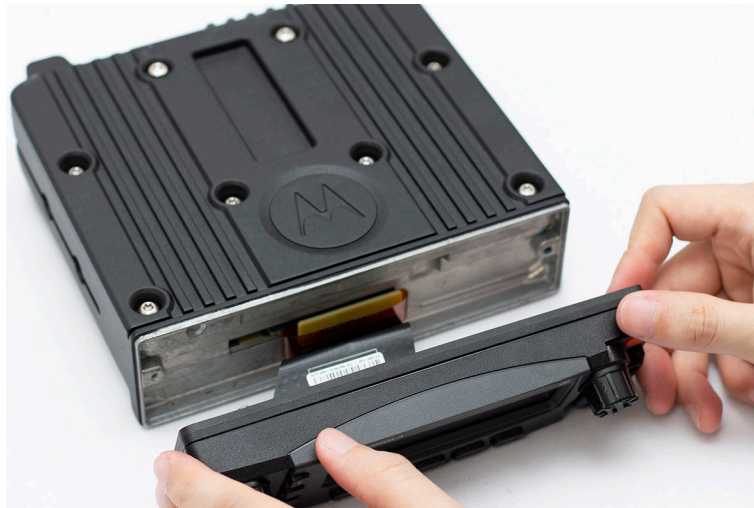
Figure 62: Removing the Control Head/TIB
