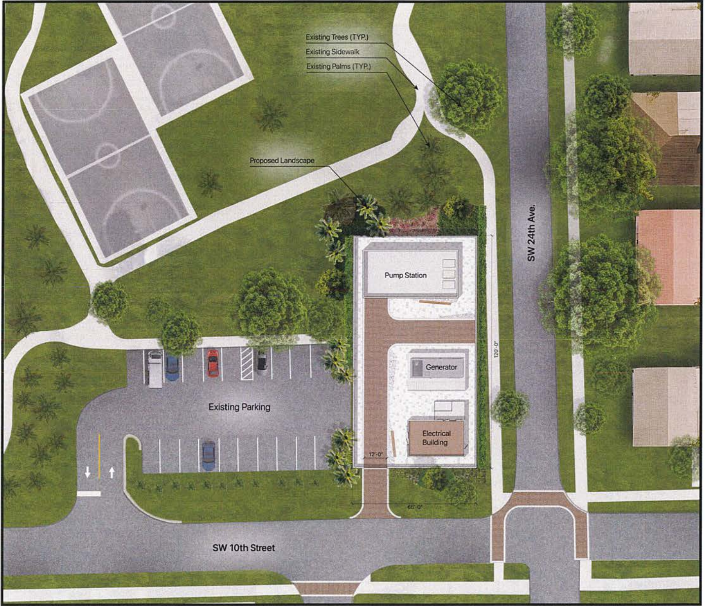
Figure 8: : Proposed Stormwater Pump Station (Riverland Park)
