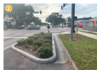
2 Floating Curb Extension in St. Petersburg, FL. Source: Alta Planning + Design
