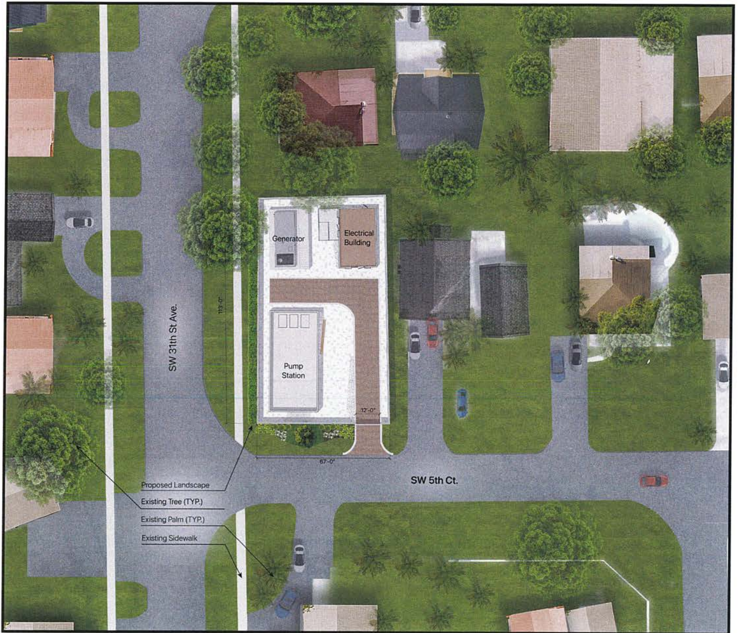
Figure 10: : Proposed Stormwater Pump Station – Option 3 (City Property)
