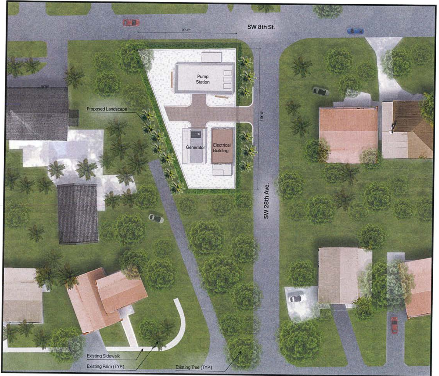
Figure 8: Proposed Stormwater Pump Station – Option 1
