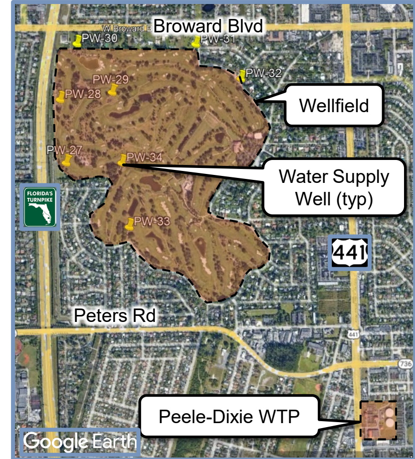
Dixie Wellfield Supplies the Peele-Dixie WTP
