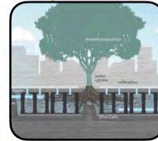
Resiliency - Silva Cells for Stormwater Management
