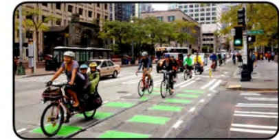
Cycle Track Dashed Intersection Markings Style
