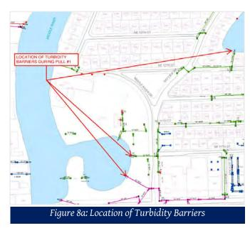
prepared by Terracon Consultants and using FDEP's Best Management Practices (BMPs). Based on preliminary review of the City's Atlases, we have identified that the storm water system located along Bayview Drive, discharging to the Middle River and Intracoastal Water Way. For the first HDD Pull (Pull #1) we have identified two 24-inch outfalls at the George English Park discharging to the Middle River and an 18-inch outfall discharging to a canal just north of NE 12<sup>th</sup> Street.
