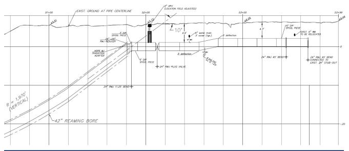
Figure 5 – Open Cut Tie-In Profile (Refer to Conceptual Plans)
