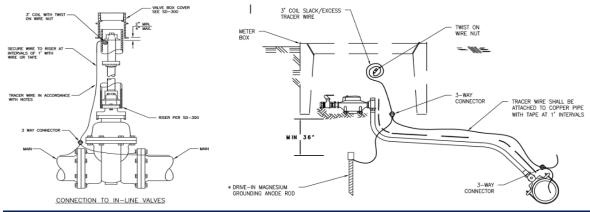
Figure 6 – Tracer Wire Installation Examples
