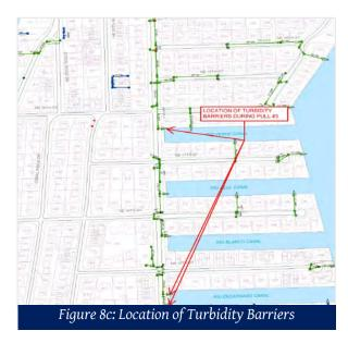
Turbidity barriers as shown in Figure 8 will be installed at these locations as the last line of defense to prevent any groundwater from reaching the water bodies.
