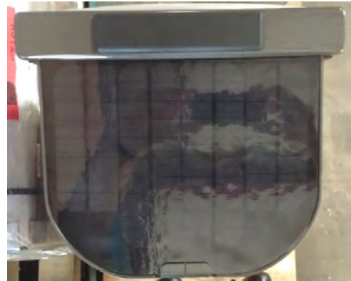
Figure 19 - Integrated solar panel on the top of the MacKay Tango™
