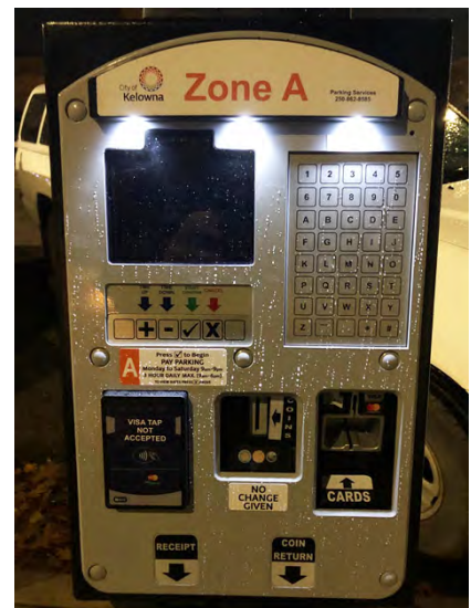
Figure 27 - Faceplate of Tango with optional LED brow light installed for dark hours
