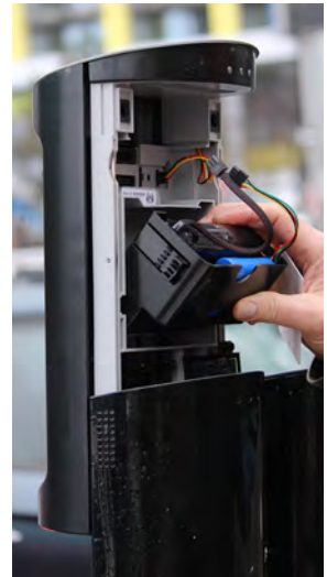
Figure 4 - Maintenance friendly access for on-street servicing
