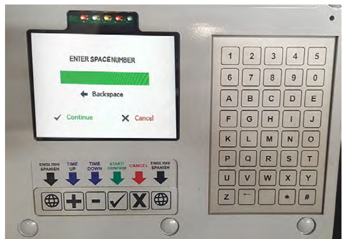
Figure 22 - Tango 6 button keypad below display screen and alphanumeric keypad to the right
