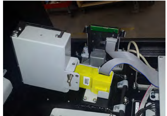
Figure 24 - Easy access to yellow Smartchute™ that can be cleaned or replaced in seconds. Same as coin chute in most MacKay single space meters.
