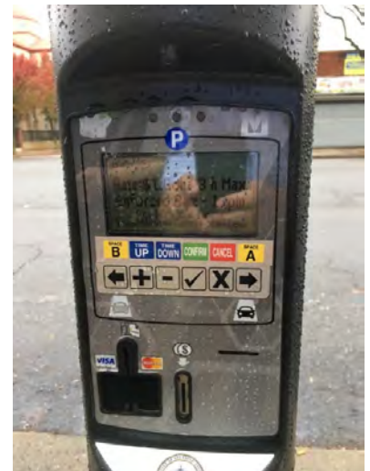
Figure 13 - mkBeacon Piezo control buttons (shown on 2-Bay mkBeacon monitoring 2 spaces)
