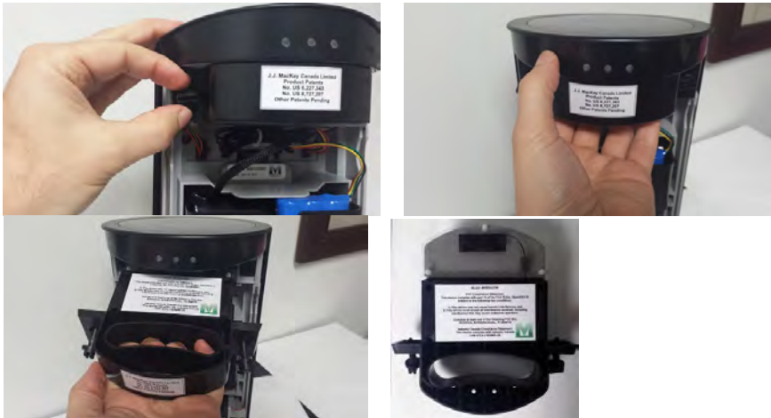
Figure 12 - mkBeacon communications module - easily removed and replaced
