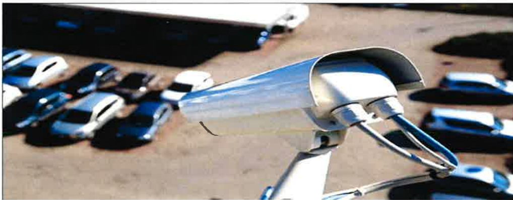
Camera covering multiple parking spaces to provide real-time occupancy information and security
