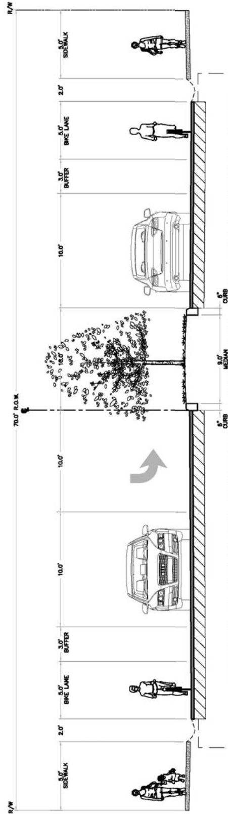
PROPOSED CONCEPTUAL TYPICAL SECTION N.E. 15TH AVENUE FROM N.E. 11TH STREET TO N.E. 12TH STREET N.T.S.
