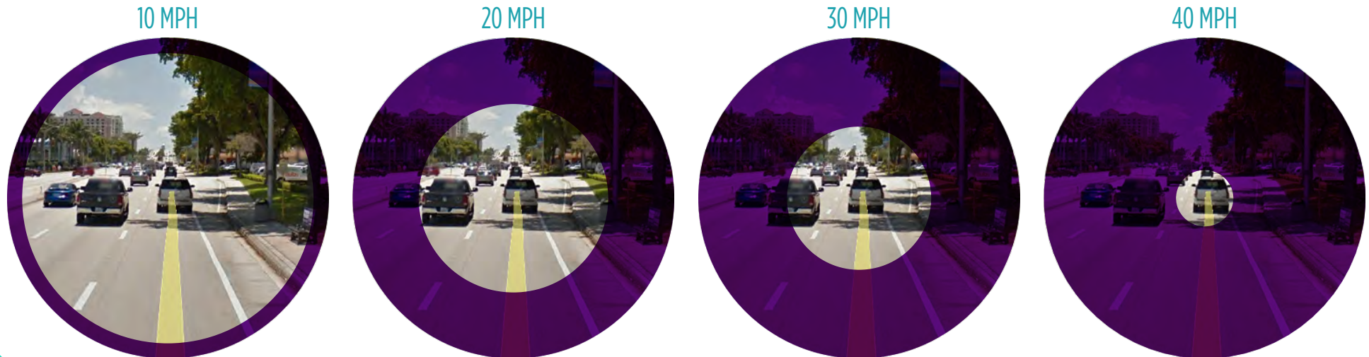
Figure 27 | Driver's Cone of Vision by Travel Speed
