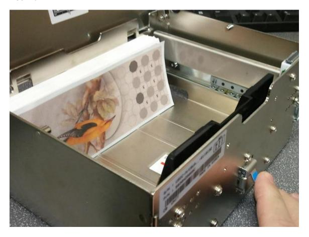
9) Drop the bills in the cassette as you see here(test media is shown). Press the blue button to release the pressure plate onto the bills, as shown in Figure 6. Make sure bills are not descending from the feed slot in the front of the cassette, as shown in Figure 7.
