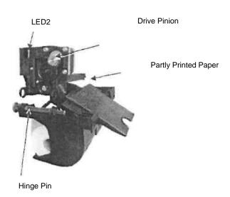
Fig. 6 Tilt the printer mechanism open for paper removal
