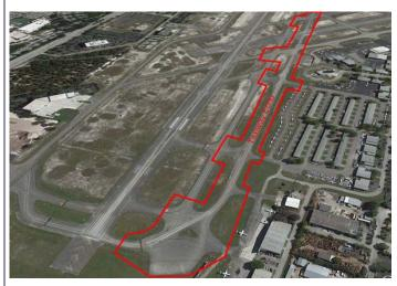
The FXE Taxiway Echo project needed to address failing pavement conditions and update geometry to comply with the FAA AC 15/5300-13A-Change 1. Taxiway Echo is the secondary parallel taxiway serving runway 9-27 nearly 6,200 feet long and 50' wide.
