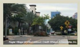
A small circular island used in the middle of intersections to force vehicular traffic to slow and negotiate around it. They also increase vehicular safety. It may be landscaped and may have mountable curbs. Raised intersections may be used in place of mini roundabouts, if desired, but may not be as effective at traffic calming.
