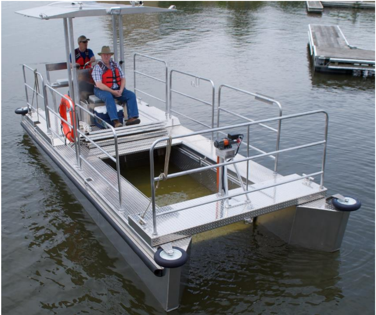
TRASH COLLECTION BASKET LOWERED IN THE WATER
