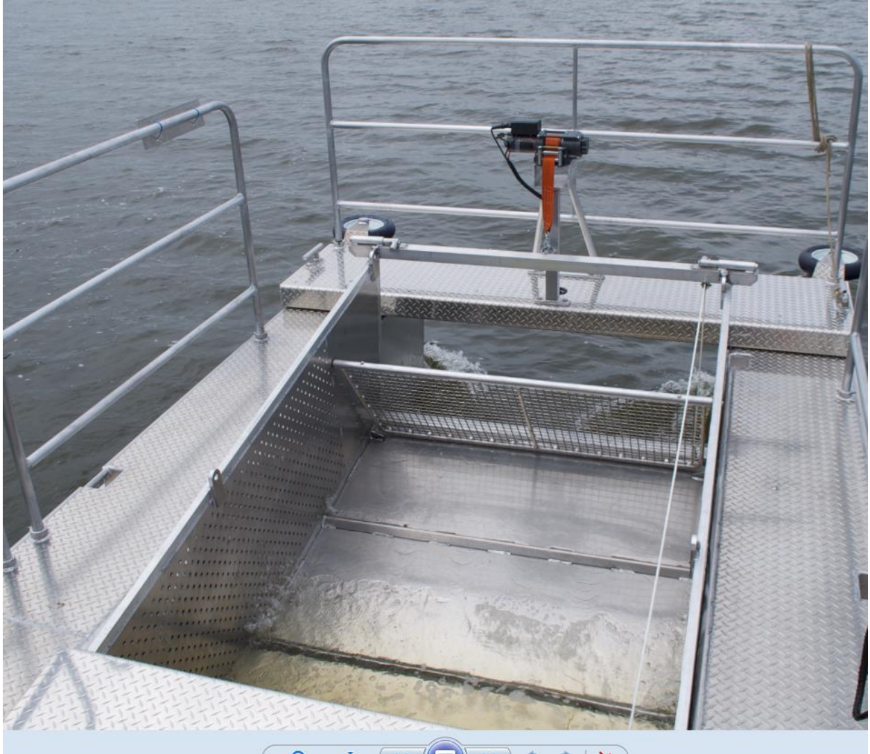
TRASH COLLECTION BASKET RAISED OUT OF WATER
