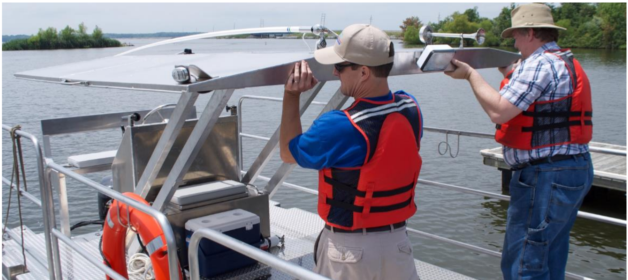
CANOPY CAN BE LAID DOWN TO REDUCE HIGHT, ENABLING PASSAGE UNDER LOW BRIDGES.
