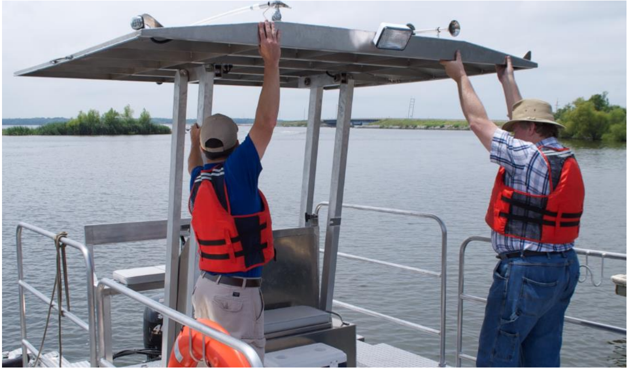
CANOPY CAN BE LAID DOWN TO REDUCE HIGHT, ENABLING PASSAGE UNDER LOW BRIDGES.
