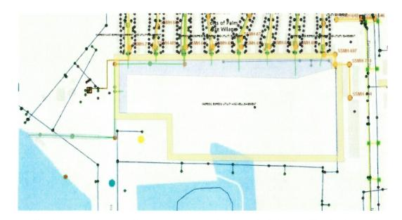
**RESPONSE:** The City's Public Works Department and Stormwater Operations determined that an easement 20'x50' would need to be dedicated to cover the existing 36' stormwater pipe that crosses the easement.
