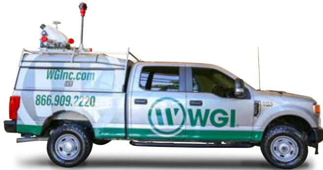
WGI's Terrestrial Mobile LiDAR Vehicle for LiDAR and Imagery Collection
