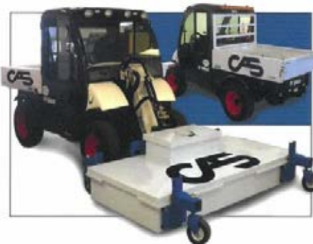
Typical 3-D Radar Tomography Scanning Unit
