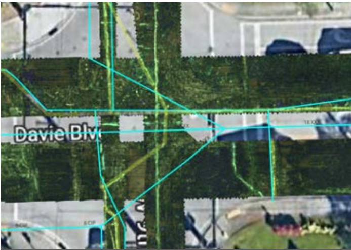
3DHS-GPR Raptor Data and Overlay of Existing GIS Vector Data Before Adjustment
