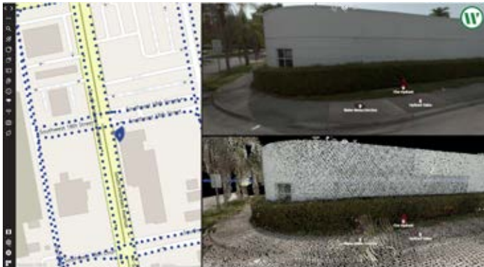
Survey-grade LiDAR and imagery of above-ground water system assets
