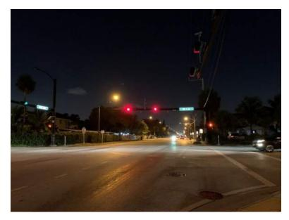
Figure 3 Davie Boulevard does not meet uniformity ratio criteria based on the review on July 22, 2021.
