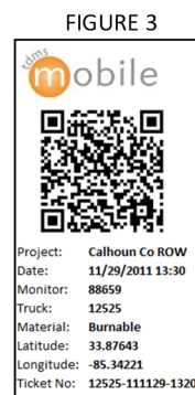
FIGURE 3 Paper tickets are created with encrypted QR code to transmit information/data.
