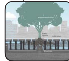
Resiliency - Silva Cells for Stormwater Management
