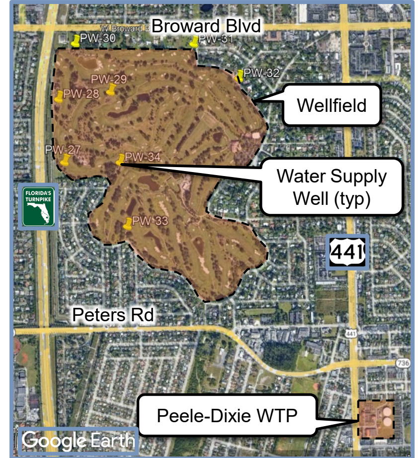
Dixie Wellfield Supplies the Peele-Dixie WTP
