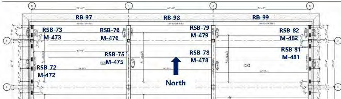
Figure 3. Plan view of structural framing at roof at north end of building (from precast shop drawings Sheet S-3A-PL dated August 16, 2022). Annotations in blue by WJE including structural drawing (top) and precast shop drawings (bottom) beam designations. Area of affected framing is generally at and north of gridline 2.
