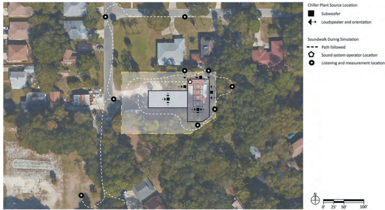
Figure 12. Aerial map showing the path (dashed line) taken during the simulation of the chiller plant. The location of the chiller building and cooling towers are shown for reference. A total of nine listening locations are indicated by the circles on the map. Sound levels from insect noise and air conditioning units operating during the times measurements were made at these locations resulted to be within -3 to +8 dB in a sound level difference when compared to the computer model.
