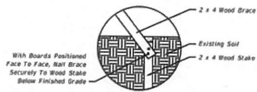
Figure 3 TREE AND PALM STAKING FOR 3" AND GREATER
