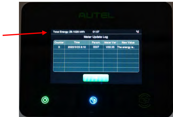
Figure 4. Event logger screen is shown on the EVFS. The totalizer is indicated by the red arrow
