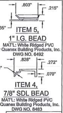
ITEM 4, 7/8" SDL BEAD MAT'L: White Ridged PVC by Quanex Building Products, Inc. DWG NO. 8483
