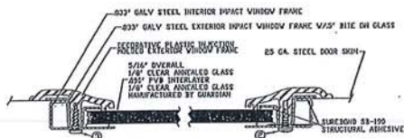
SECTION B-B IMPACT WINDOW DETAIL N.T.S.
