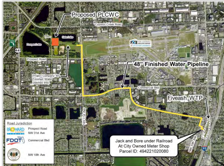
Figure 2-8: Finished Water Pipeline from PLCWC to Fiveash
