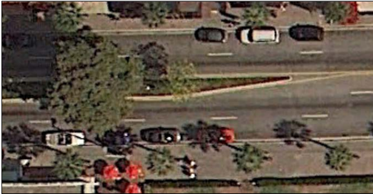
On-street parking west of 8th Avenue Limits Throughput
