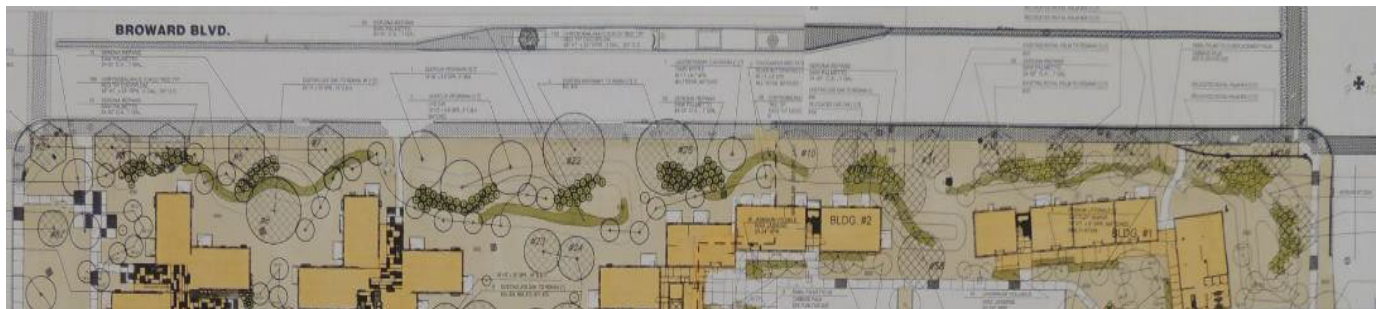
The Kennedy Homes Landscape Plan for the streetscape along Broward Boulevard meets the current 50-50% Tree/Palm requirement
