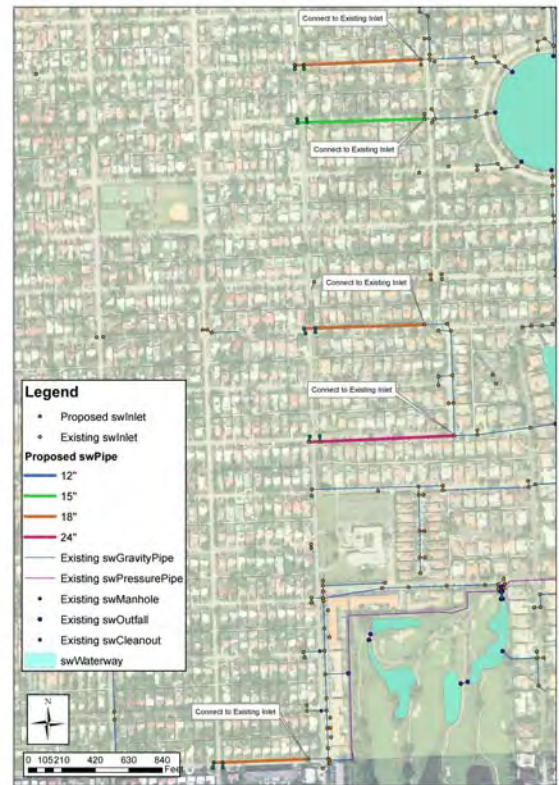
Drainage System Extension
