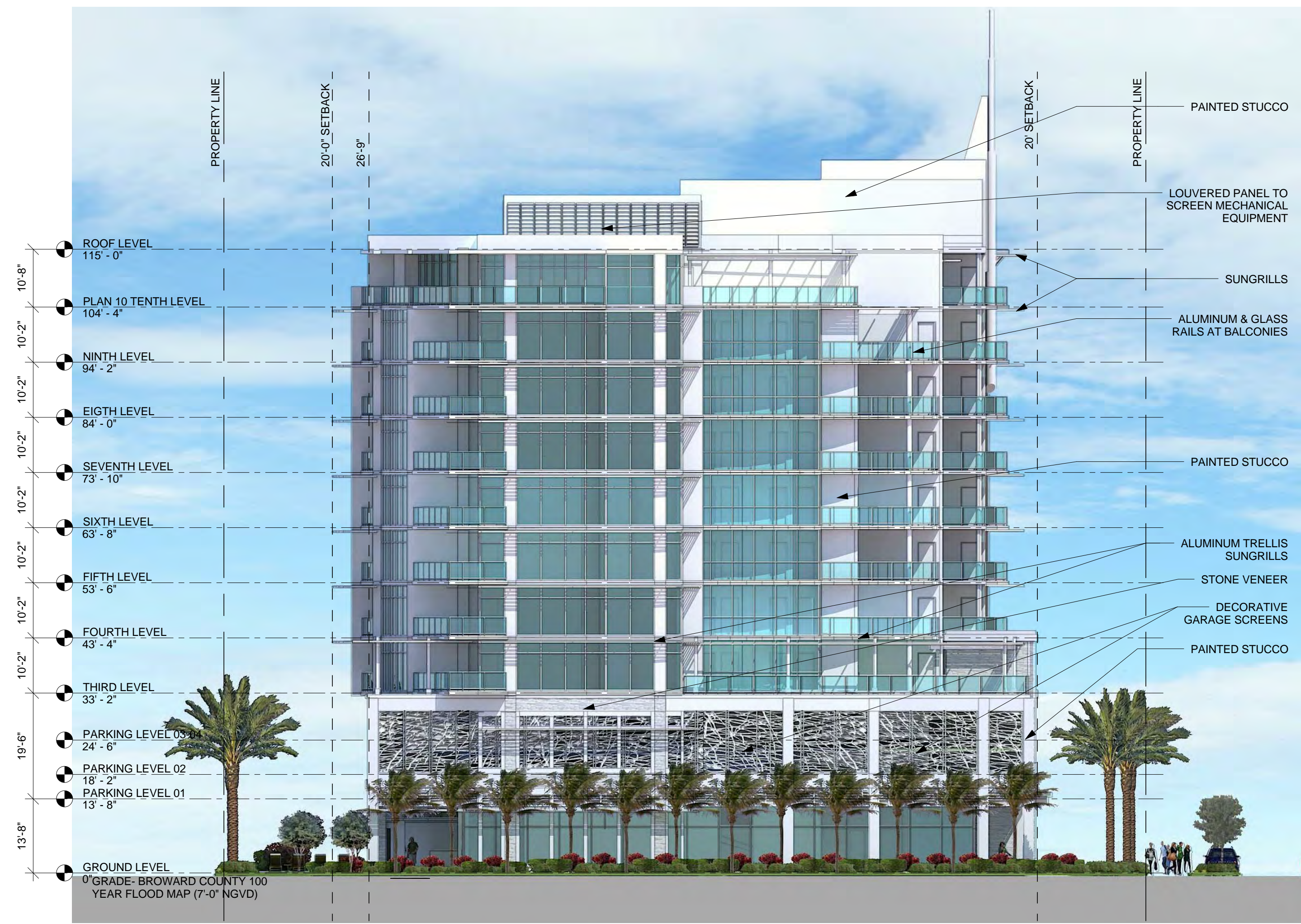
SOUTH EAST ELEVATION 4 1/16" = 1'-0" A-2.01
