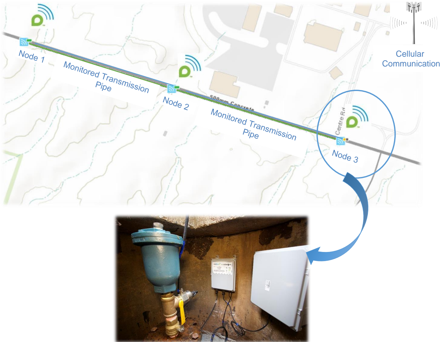
Figure 8: EchoShore®-TX Configuration spaced approximately every half mile along a transmission pipe – Each monitoring node fits comfortable inside a standard chamber
