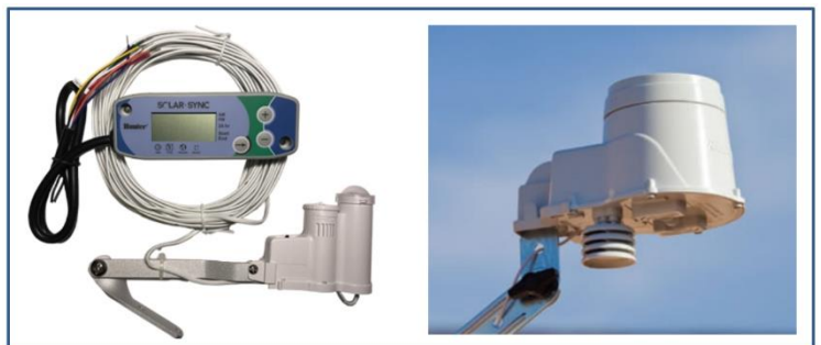
Figure 2b. On-site weather sensing pods. These pods contain several sensors measuring weather and climate conditions. Information is then sent to the controller, which 'knows' the general characteristics of the landscape and soil. Irrigation timing and volumes are then adjusted to meet, but not exceed, plant needs.
