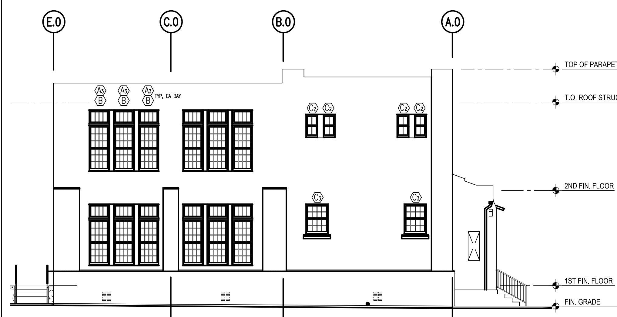
3 NORTHWEST ELEVATION - PROPOSED SCALE: 1/8" = 1'-0"
