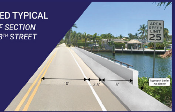
Fig. 4 – No approach railing at ends of bridge 865765
