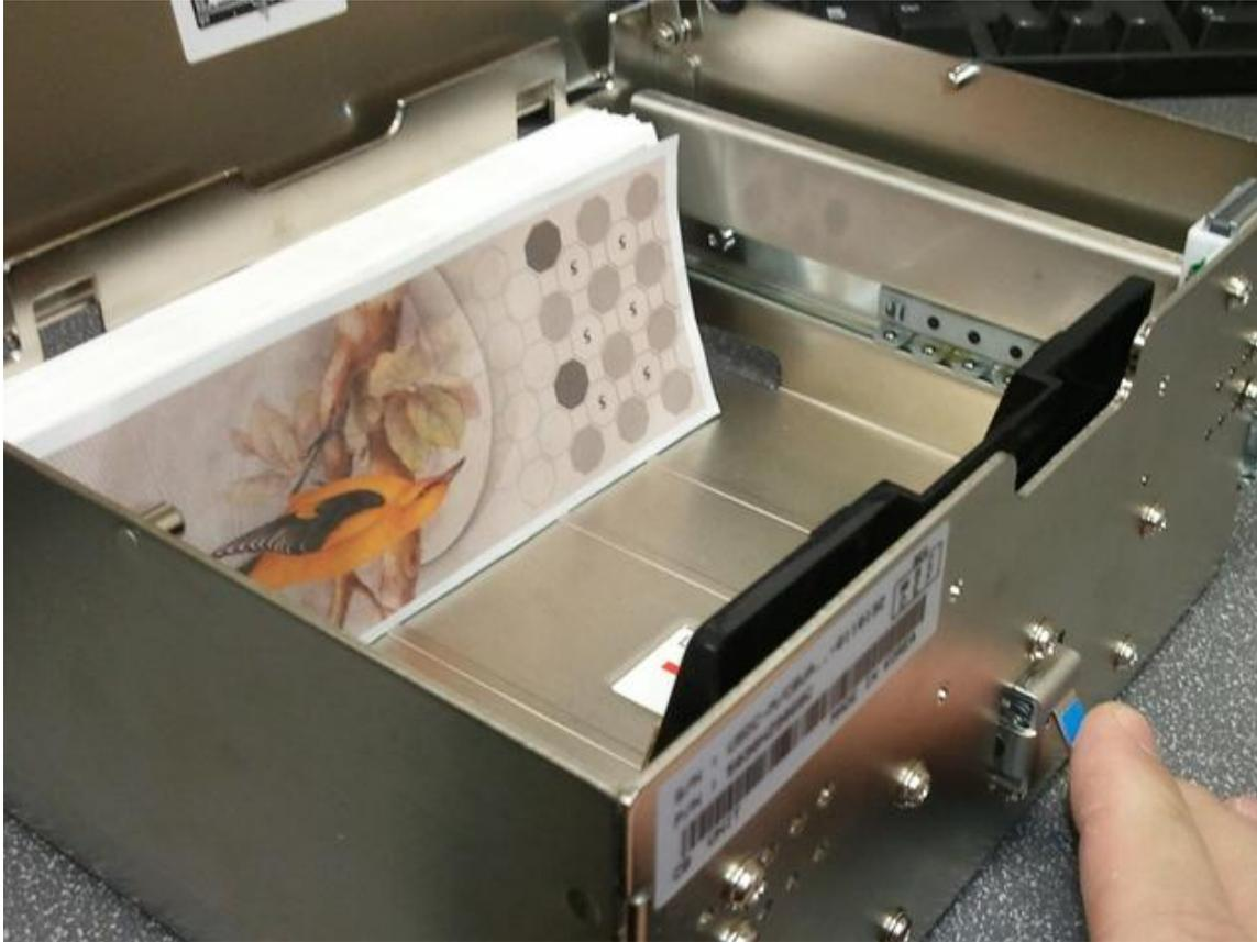
9) Drop the bills in the cassette as you see here(test media is shown). Press the blue button to release the pressure plate onto the bills, as shown in Figure 6. Make sure bills are not descending from the feed slot in the front of the cassette, as shown in Figure 7.
