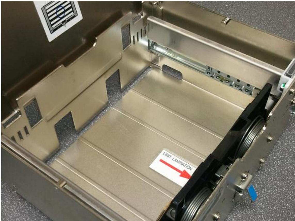
8) Open the cassette by pulling back the spring loaded pressure plate until it clicks. Load bills as shown in Figure 6. When loading new bills, make sure to flip through the bills so they're not sticking to each other, flex them and shuffle them a few times. This will minimize dispense errors and rejected bills.
