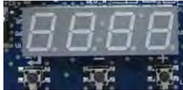
The motor control board contains a four-digit, seven-segment display that is used to present information in a format close to real-world language, while having a small-form factor. Most characters are immediately recognizable; however, please consult [Table 17](#) and [Table 18](#) for the graphical representation of each alphanumeric character.
