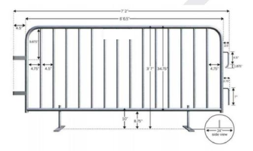
Interlocking hook & sleeve system for security and safety
