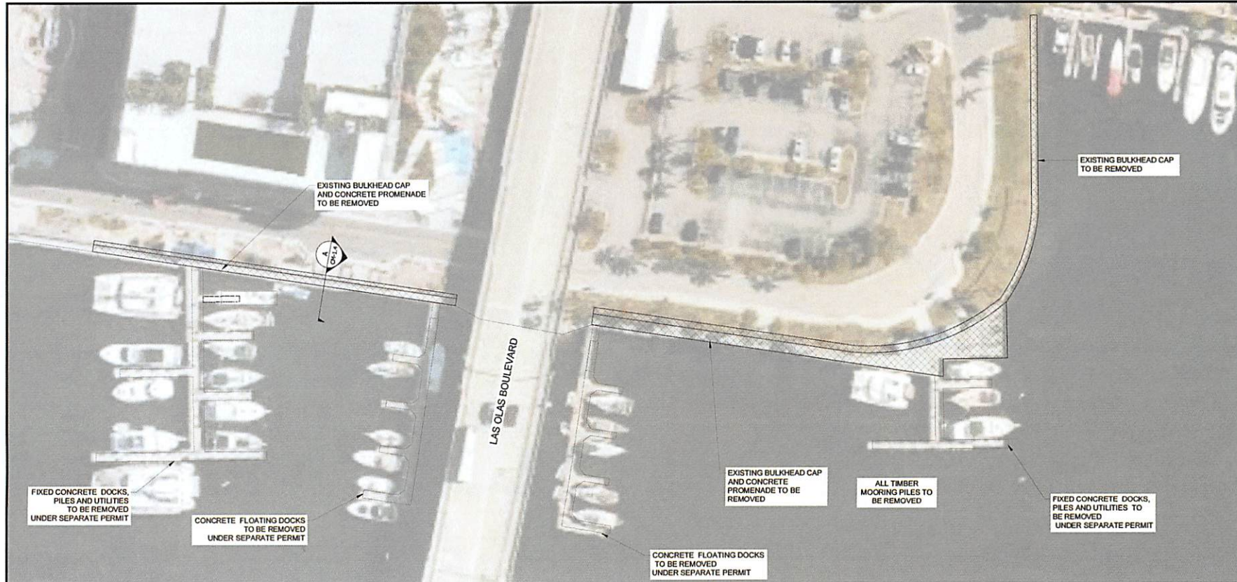
DEMOLITION PLAN SCALE: 22X34 1" = 20' 11X17 1" = 40'
