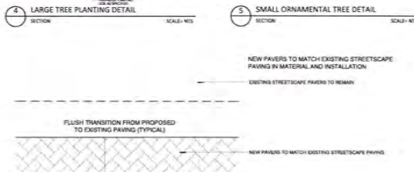
9 WALKWAY / PLAZA PAVING ENLARGEMENT SCALE: NTS
