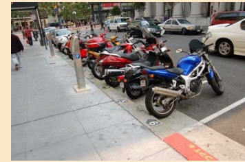
[Figure 4.252] Parking for mopeds and motorcycles can be combined with standard parking for vehicles.
