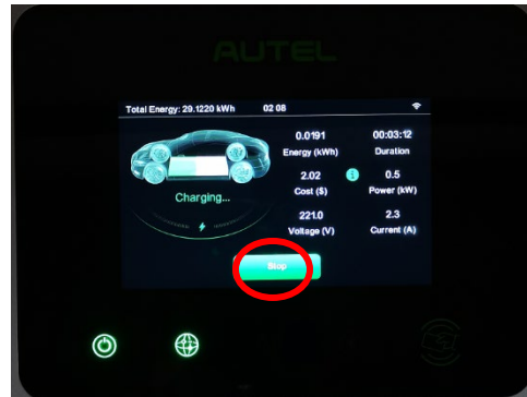
Figure 5. Charger screen active charge session stop button
