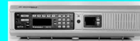
Backup Control Station
