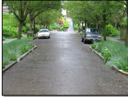
Curb Extensions with infiltration (rain gardens)
