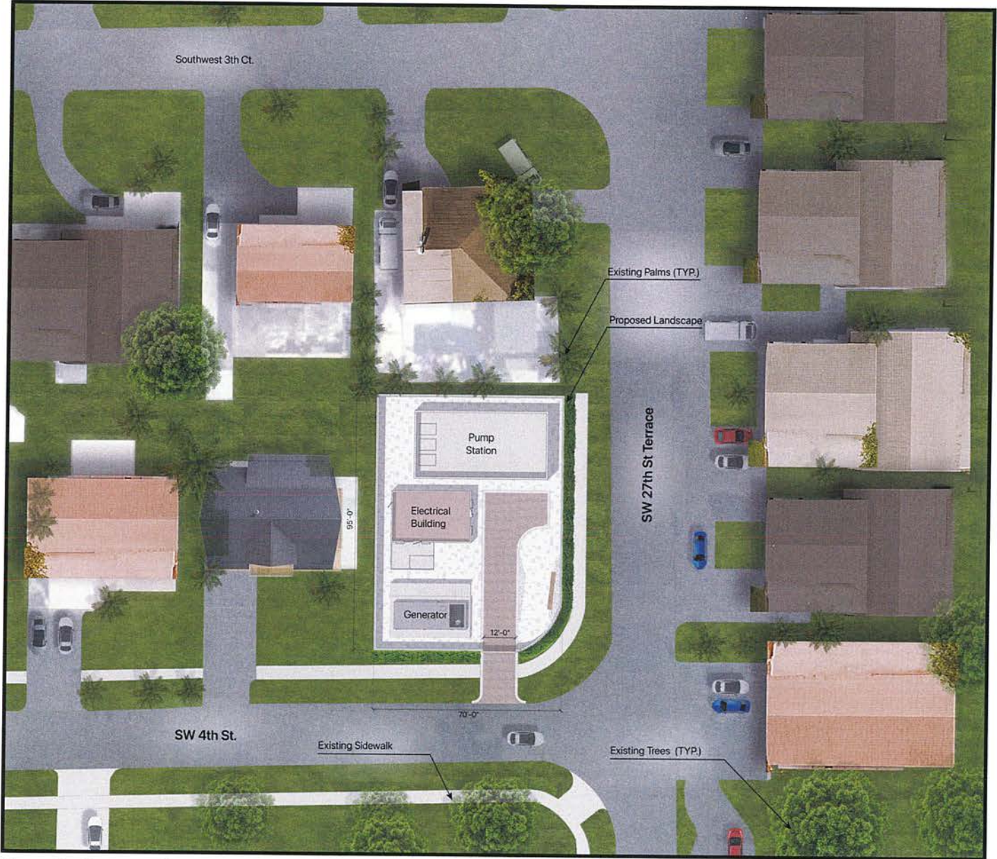
Figure 9: : Proposed Stormwater Pump Station – Option 2
