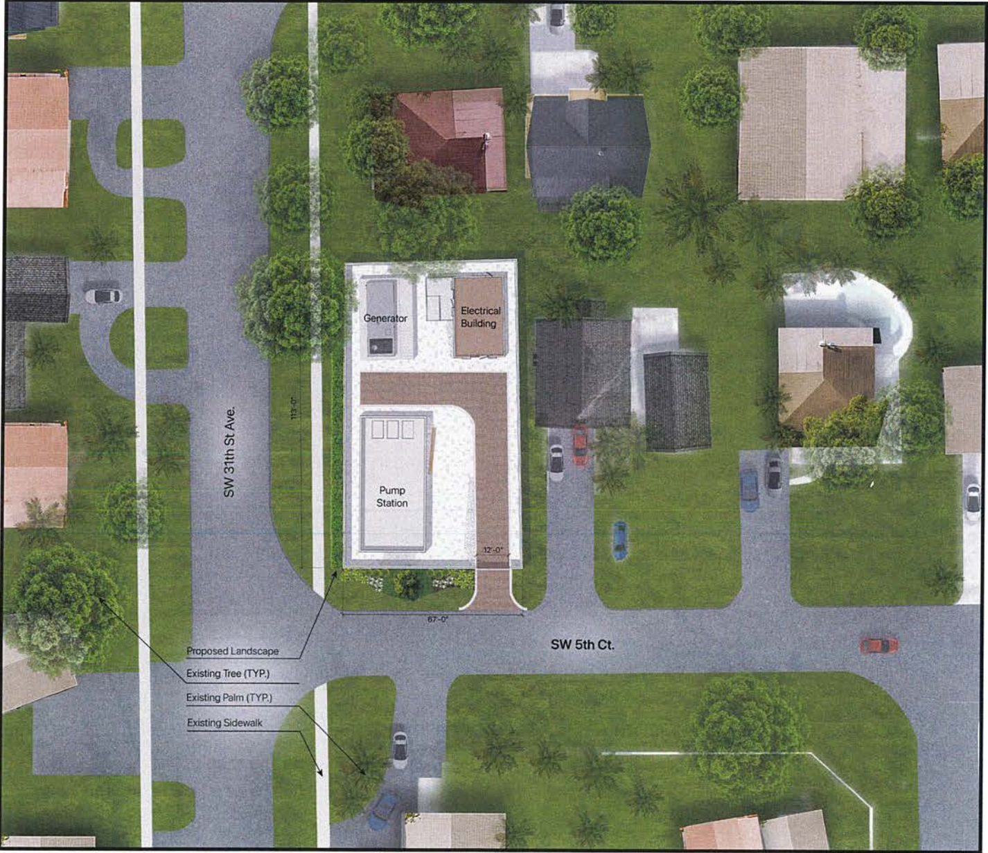
Figure 10: : Proposed Stormwater Pump Station – Option 3 (City Property)
