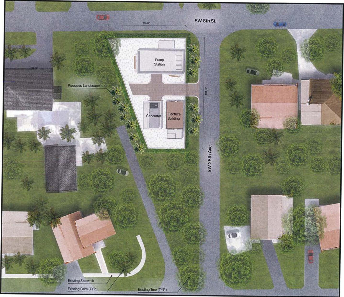
Figure 8: Proposed Stormwater Pump Station – Option 1
