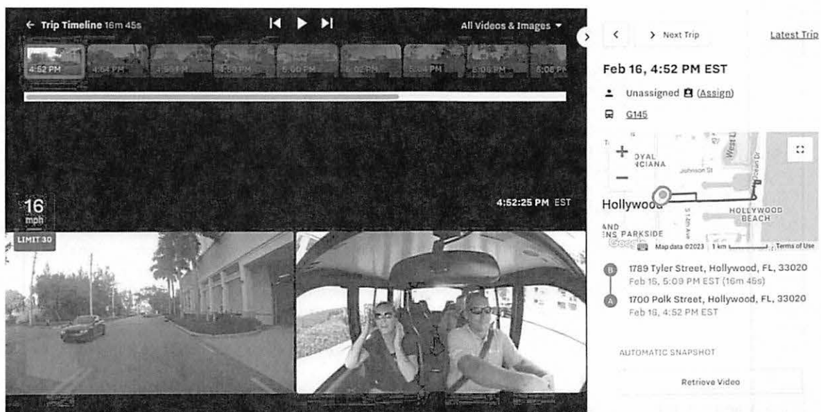
Samsara AI Dash Cam dashboard with both views, saved footage and trip details including trip route, duration and pick-up and drop-off locations.
