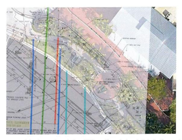
Approximate pile locations are shown in the aerial above with a project overlay indicating the expected locations of the utilities within the easements. We have not been told the depth of the force main utility (shown as a green line) that is located within the easement with the FPL utility (shown as a red line). Based on the aerial, the distance from the two closest piles appears to be 12-15 feet to the force main and 27-30 feet to the FPL line.
