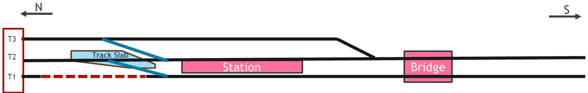
The above diagram depicts that, at this stage, Track T1 north of the track slab can be completely taken out of service it North of the station. Nevertheless, the station will continue to operate as usual, as it remains accessible via Track T2 and Track T3. Also, the bypass track T3 remains operational.
