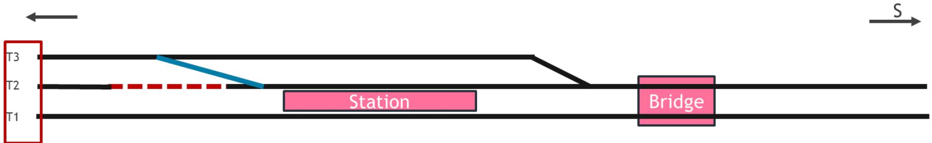
The above diagram depicts that Track T2 is taken out of service to allow the installation of track slab at this location, while the station and the bypass tracks remains operational due to the presence of Track T1 and Track T3, which can be used to access the crossover and the station.
