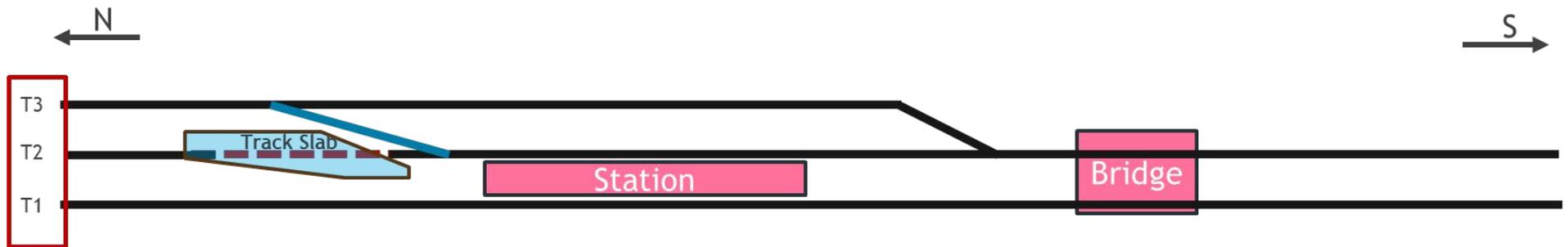
The above diagram depicts the construction of the track slab in this area. The track slab will be a structural slab that will be placed on the ground once the track is removed. Its purpose is two-fold:
