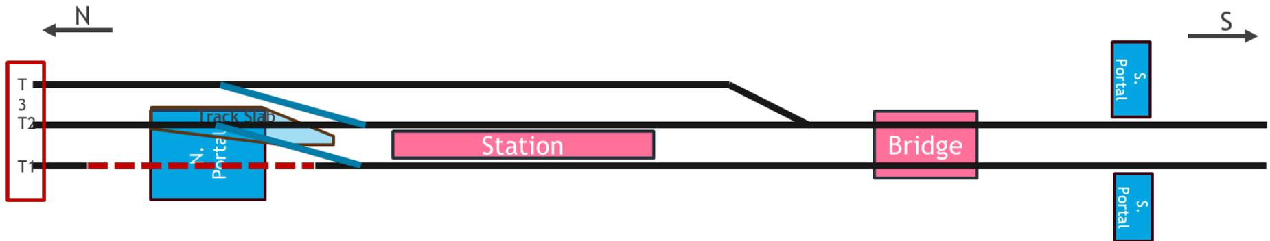
The above diagram depicts that construction will take place from the North at this location. Beneath the existing track slab/decking and the removed track, the North portal will be built, along with the launching shaft for the TBM. Simultaneously, towards the South direction, the two portals required to receive the TBM will also be constructed.
