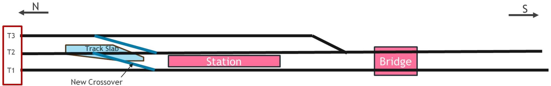
The above diagram depicts the installation of another crossover between Track T2 and Track T1 to allow rail operation flexibility. The track slab acts as a foundation for Track T2 and as roof slab for future cut-and-cover portal.
