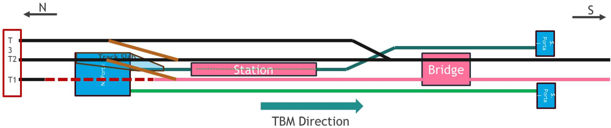
The above diagram depicts the TBM is taken from the south portal and relocated to the same launch shaft area in North portal for subsequent launches from north portal. The green indicates the direction of the TBM, the black indicates the surface tracks, while the blue represents the path towards the South portal where it can be retrieved.
