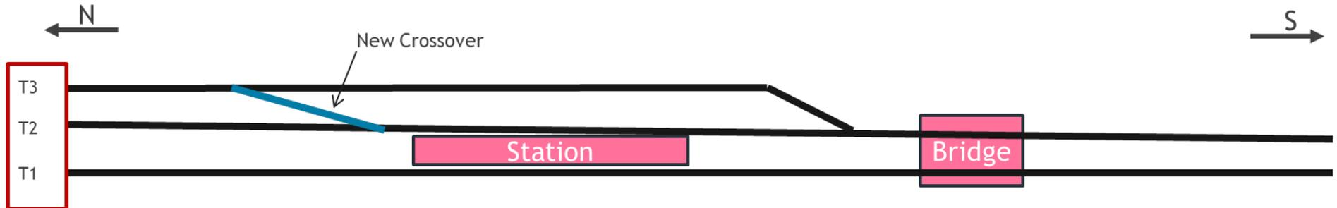
The above diagram depicts the initial step that involves installing a crossover between Track T3 and Track T2. This allows the flexibility of rail operation to connect to the station or to bypass the station as needed.
