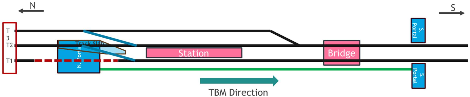
The above diagram depicts that the objective is to have the first run of the TBM between by launching TBM from the North. Note that the green is a tunnel while the black are surface tracks.
