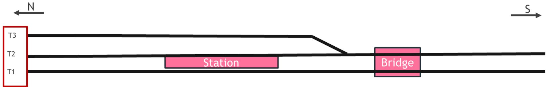
The diagram above, depicts how the process of maintaining operational tracks involves construction sequencing. When examining the actual tunnel, more data will likely be gathered. The diagram is schematic and not to scale but rather illustrates how the railroad remains functional during this type of work. Essentially, it represents the current state where there is a bridge and a station, with a surface track just before the station that can be used to bypass it.
