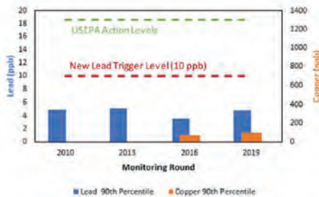
In addition to historical 90th percentiles for lead and copper, we will examine min., max, 25th, 50th and 75th percentile and site-specific trends to assess current CCT performance and potential compliance concerns with the lead action or trigger levels, if sufficient data are available.
