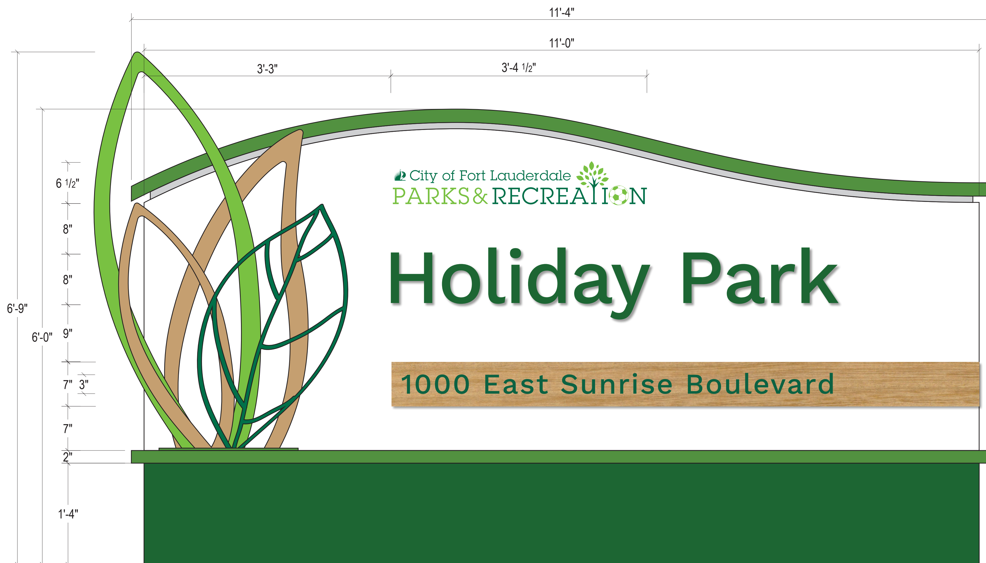
SIGN TYPE A1-C ELEVATION VIEW
